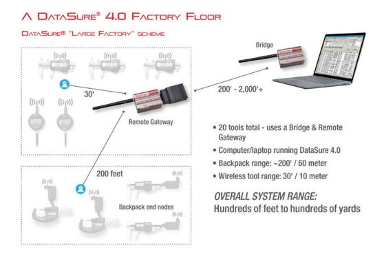
And in an "Enterprise Scheme", measurement data transmission can be increased from hundreds of yards to over a mile. By using remote gateways, bridges and perhaps adding in repeaters, over 100 measuring tools can be incorporated. Each remote gateway can facilitate 20 measuring tools. For even greater distances, Yagi Long Range Antennas can be incorporated in the scheme.
