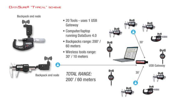
In a "Large Factory Scheme" example, 20 measuring tools can use a bridge and remote gateway to expand the total data transmission range to hundreds of feet or yards.
